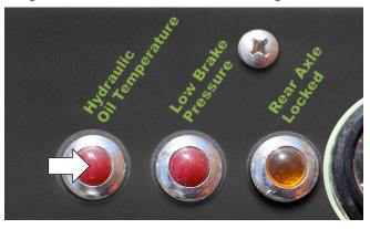
Figure 7-14. Hydraulic Oil Temperature Indicator.
