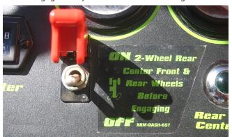
Figure 6-40. Two Wheel Rear (2WR) Steering Switch.
