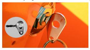
Figure 7-9. Key and Ignition Switch.
