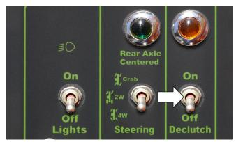
Figure 6-33. Declutch Switch.
