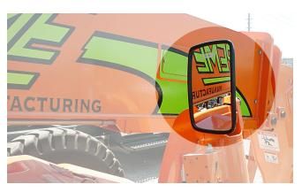
Figure 6-15. Frame Mounted Mirror.
