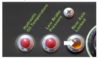
Figure 7-16. Rear Axle Lock Indicator.
