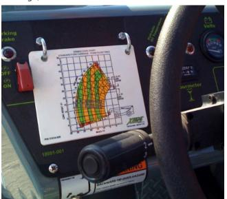
Figure 7-37. Typical Load Capacity Chart.
