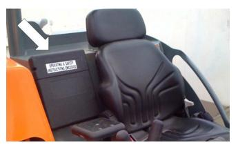
$\label{lem:continuous} \textbf{Figure 7-6. Store Operation and Safety Manual In Protective Case.}$
