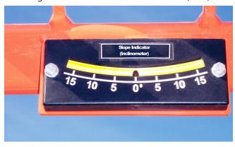
Figure 6-43. Frame Level Indicator.
