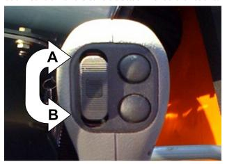
Figure 6-36. Attachment Tilt Switch.
