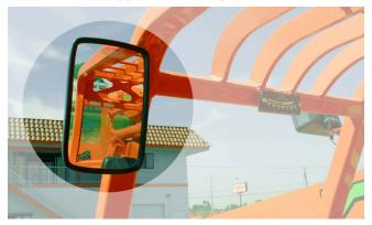
Figure 6-14. Cab-Mounted Mirror.
