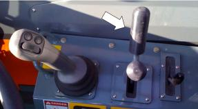
Figure 7-34. Frame Sway Control Handle.
