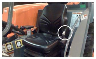
Figure 6-12. Backrest Angle Adjustment Lever.
