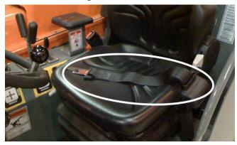
Figure 6-13. Retractable Seat Belt.
