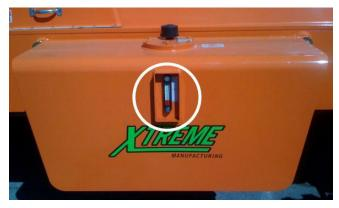
Figure 7-1. Check Hydraulic Oil Sight Gauge.
