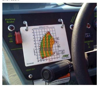
Figure 6-19. Typical Load Capacity Chart.
