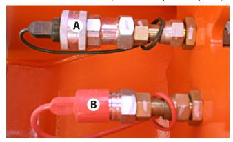
Figure 7-28. Connect Quick Attach Couplers. (A) Female Coupler. (B) Male Coupler.
