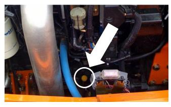
Figure 7-4. Check Engine Oil Level. Add Engine Oil, If Necessary.
