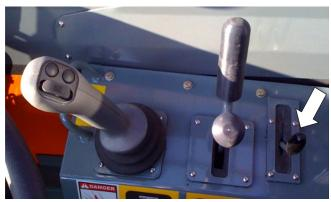
Figure 7-19. Auxiliary Attachment Control Lever.
