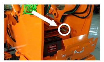
Figure 8-5. Battery Disconnect Switch.
