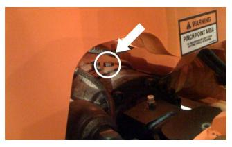
Figure 2-1. Brake Release Bolt A.
