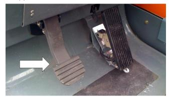
Figure 6-5. Service Brake Pedal.
