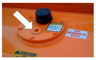
Figure 7-2. Add Hydraulic Oil, If Necessary.
