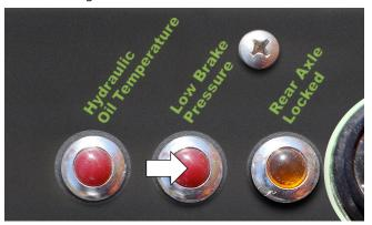
Figure 7-15. Low Brake Pressure Indicator.
