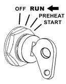
Figure 7-12. Ignition Switch Automatically Returns To RUN.
