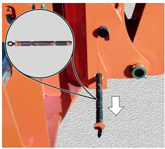
Figure 7-31. Pull Quick Attach Pin from Attachment and Quick Attach Adapter.
