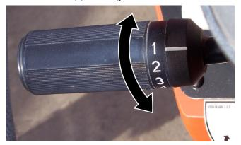
Figure 6-17. Gear Select Switch.
