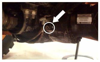
Figure 2-2. Brake Release Bolt B.
