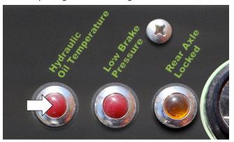
Figure 6-20. Hydraulic Oil Temperature Indicator
