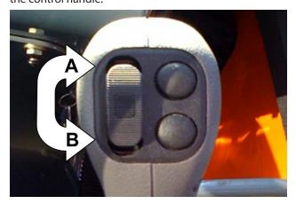
Figure 7-18. Attachment Tilt Control Switch. (A) Attachment Tilt Down. (B) Attachment Tilt Up.
