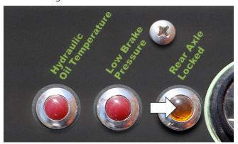
Figure 6-22. Rear Axle Lock Indicator.
