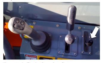
Figure 6-39. Auxiliary Attachment Control Lever.
