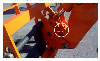
Figure 7-25. Raise Quick Attach Lock Lever.
