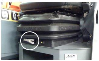
Figure 6-9. Weight Suspension Lever.
