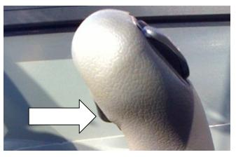
Figure 6-38. Frame Sway Override Switch.
