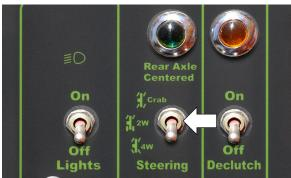
Figure 6-31. Steering Select Switch.
