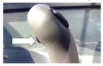
Figure 7-36. Frame Sway Override Switch.
