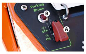
Figure 7-8. Parking Brake Switch (A) Must Be ON (Engaged) To Start The Reach Forklift.
