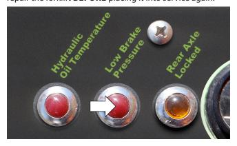
Figure 6-21. Low Brake Pressure Indicator.
