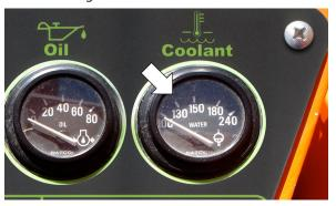
Figure 6-27. Coolant Gauge.
