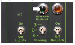
Figure 6-30. Rear Axle Centering Indicator.
