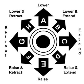
Figure 6-35. Boom Control Handle Functions.
