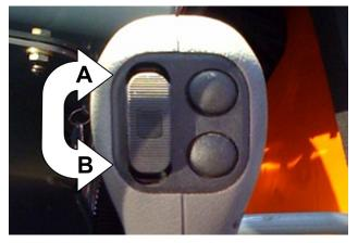
Figure 7-19. Attachment Tilt Control Switch. (A) Attachment Tilt Down. (B) Attachment Tilt Up.
