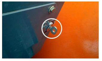
Figure 6-1. Key and Ignition Switch.
