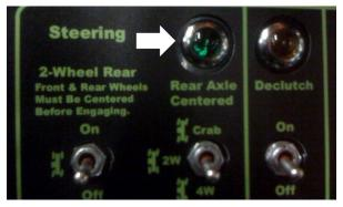
Figure 6-30. Rear Axle Centering Indicator.
