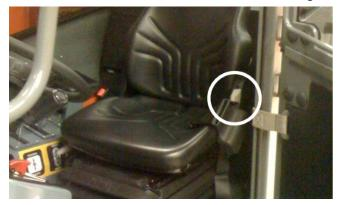
Figure 6-12. Backrest Angle Adjustment Lever.
