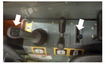
Figure 7-20. Fork Positioning Control Handle.
