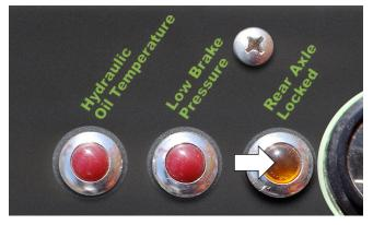
Figure 6-22. Rear Axle Lock Indicator.
