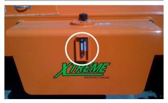
Figure 7-1. Check Hydraulic Oil Sight Gauge.
