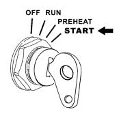
Figure 7-11. Turn Key In Ignition Switch To START.
