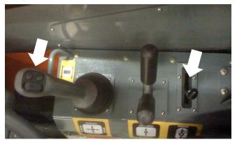
Figure 6-39. Auxiliary Attachment Control Lever.
