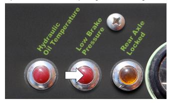
Figure 6-21. Low Brake Pressure Indicator.
