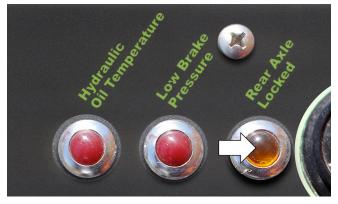
Figure 7-16. Rear Axle Lock Indicator.
