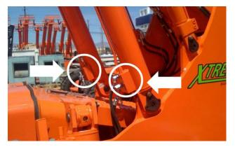
Figure 8-4. Lift Cylinder Lower Down Valve.
