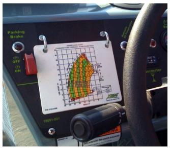
Figure 6-19. Typical Load Capacity Chart.
