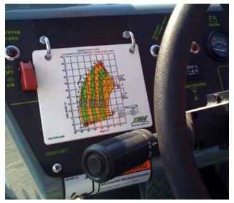
Figure 7-37. Typical Load Capacity Chart.
