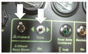
Figure 6-29. Turn Signal and Hazard Light Switches.
