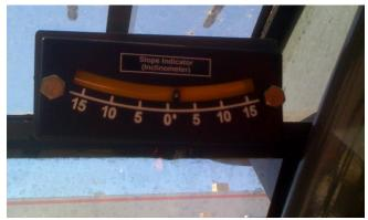
Figure 6-43. Frame Level Indicator.
