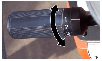
Figure 6-17. Gear Select Switch.
