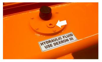
Figure 7-2. Add Hydraulic Oil, If Necessary.
