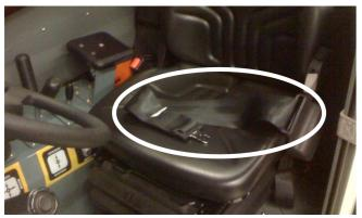
Figure 6-13. Retractable Seat Belt.
