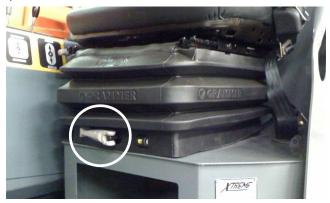
Figure 6-9. Weight Suspension Lever.
