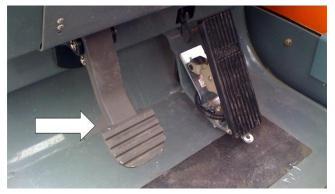
Figure 6-5. Service Brake Pedal.
