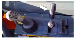
Figure 7-34. Frame Sway Control Handle.
