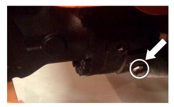
Figure 2-3. Brake Release Bolt C.
