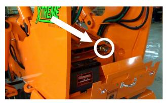
Figure 8-5. Battery Disconnect Switch.
