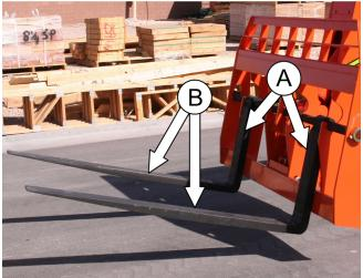
Figure 7-18. Fork Ratings. (A) Maximum Load Capacity Rating. (B) 24 Inch Load Center.
