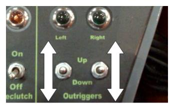
Figure 6-33. Outrigger Toggle Switches.
