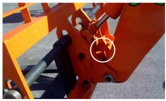
Figure 7-25. Raise Quick Attach Lock Lever.
