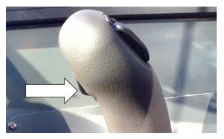
Figure 7-36. Frame Sway Override Switch.
