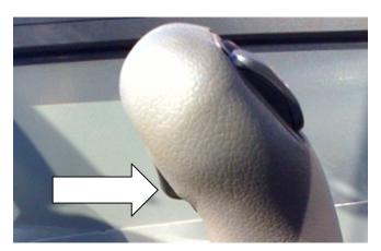
Figure 6-38. Frame Sway Override Switch.
