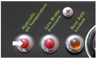
Figure 7-14. Hydraulic Oil Temperature Indicator.
