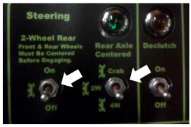
Figure 6-31. Steering Select and 2-Wheel Rear Switches.
