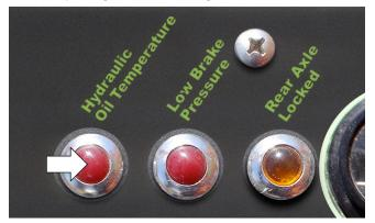
Figure 6-20. Hydraulic Oil Temperature Indicator.
