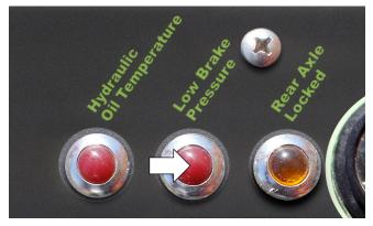
Figure 7-15. Low Brake Pressure Indicator.
