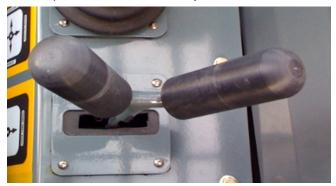
Figure 6-37. Frame Sway Control Handle.
