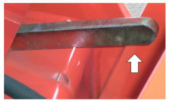
Figure 7-30. Raise Quick Attach Lock Lever.
