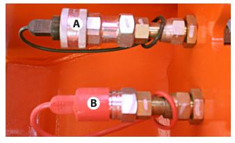
Figure 7-21. Quick Attach Couplers For Hydraulic Systems. (A) Female Coupler. (B) Male Coupler.
