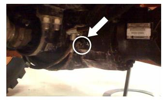
Figure 2-2. Brake Release Bolt B.
