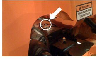
Figure 2-1. Brake Release Bolt A.
