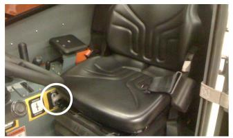
Figure 6-11. Fore and Aft Adjustment Lever.
