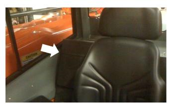
Figure 7-6. Store Operation and Safety Manual In Protective Case.
