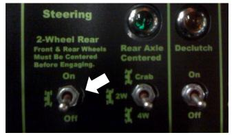
Figure 6-40. Two Wheel Rear (2WR) Steering Switch.
