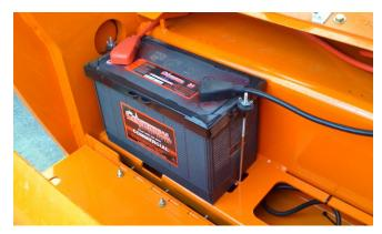
Figure 7-5. Check Battery Case and Terminals.
