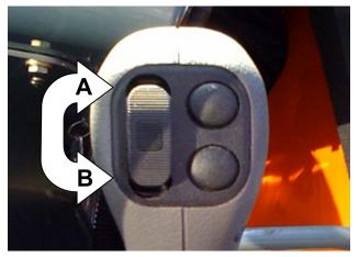
Figure 6-36. Attachment Tilt Switch. (A) Attachment Tilt Down. (B) Attachment Tilt Up.
